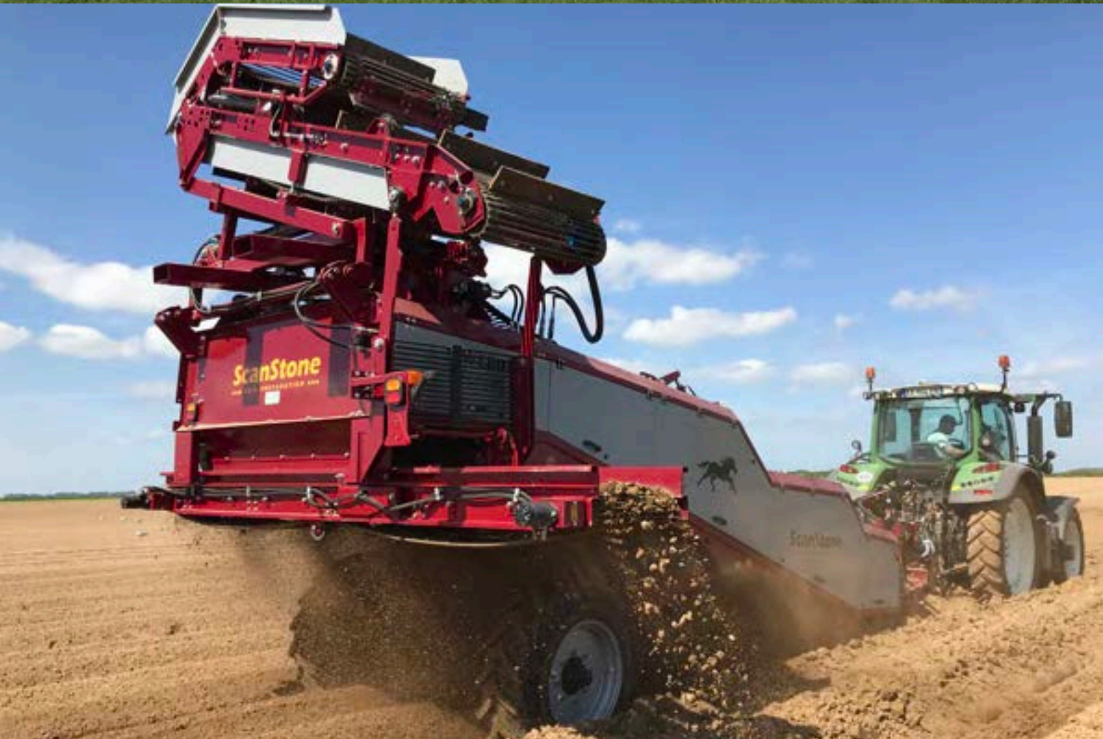
STONE HARVESTING ELEVATOR
